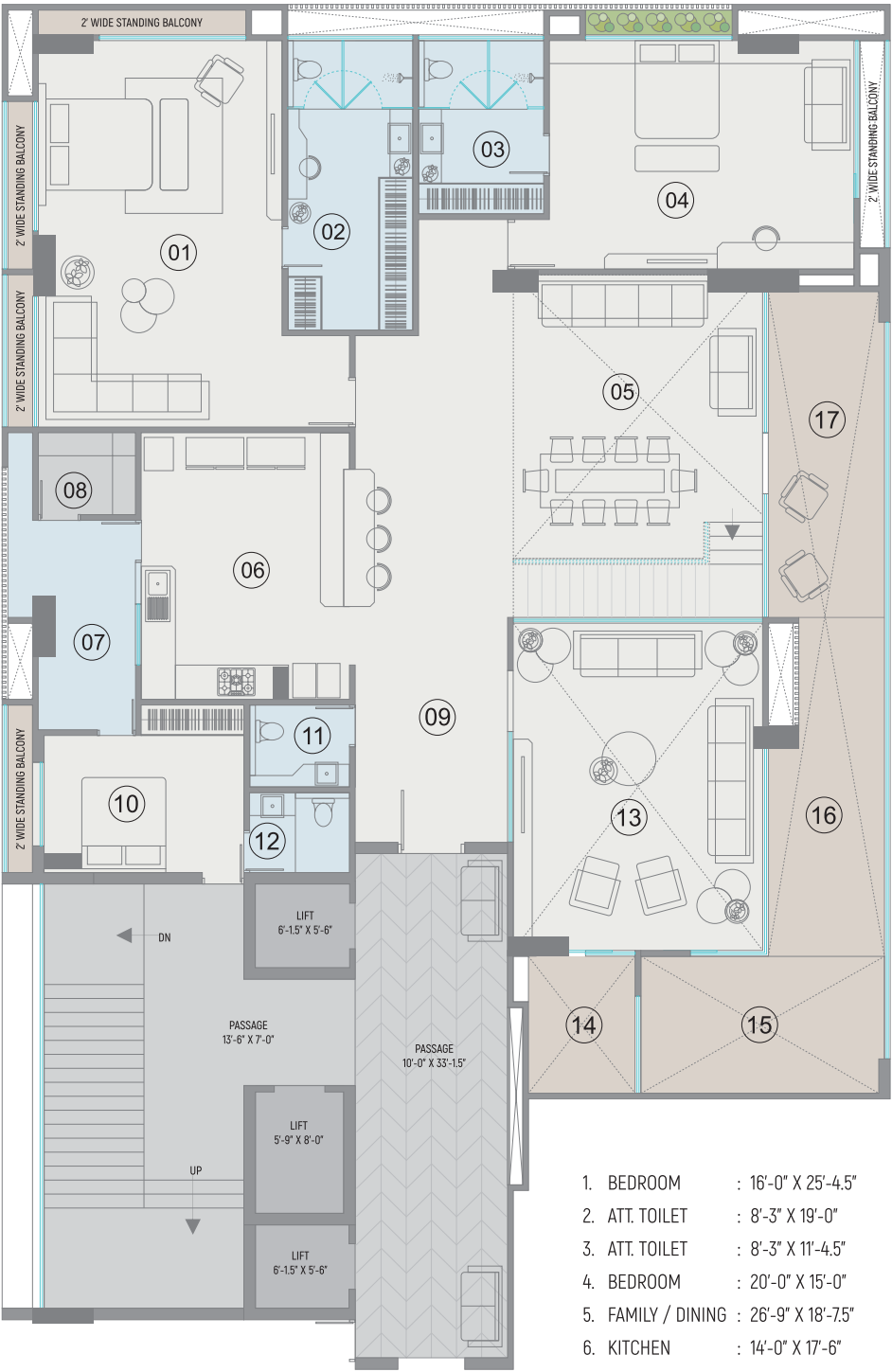
12th floor plan (penthouse lower level)
